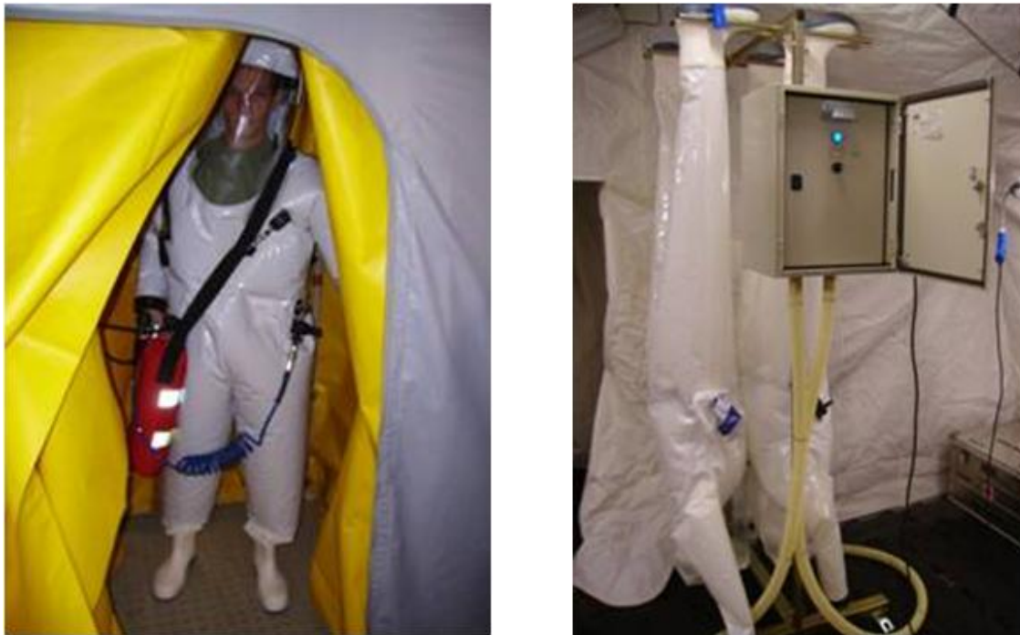
Figure 2-3: The Hygienic Section of the Deployable Biological Laboratory.
