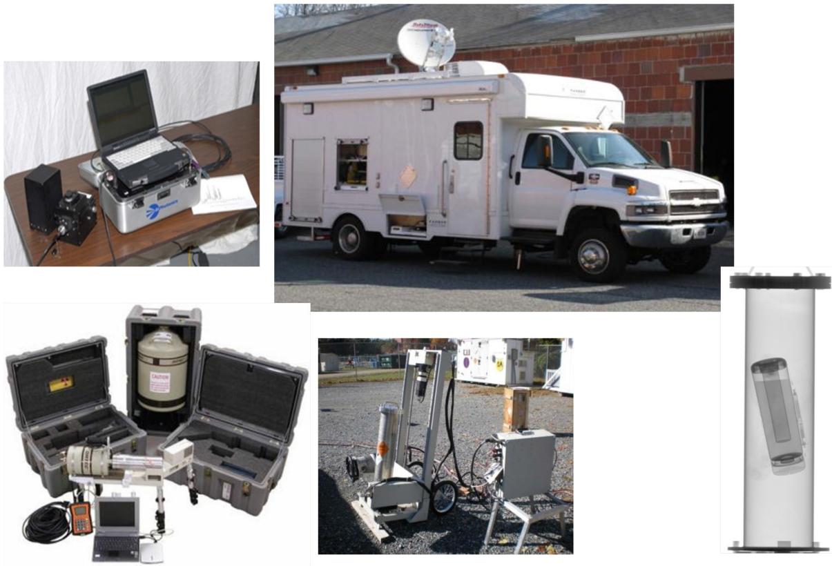
Figure 6-2: Pictures of the Mobile Munitions Assessment System (from Top Left to Bottom Right): RAMANS Spectrophometer; MMAS Phase 2 System 2; Portable Isotopic Neutron Spectroscopy System; Digital Radiography / Computed Tomography.
